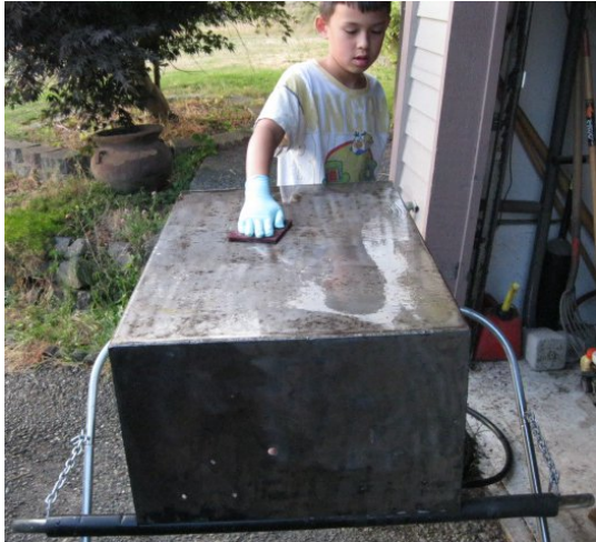
Scrubbing bare metal with water/vinegar mixture
