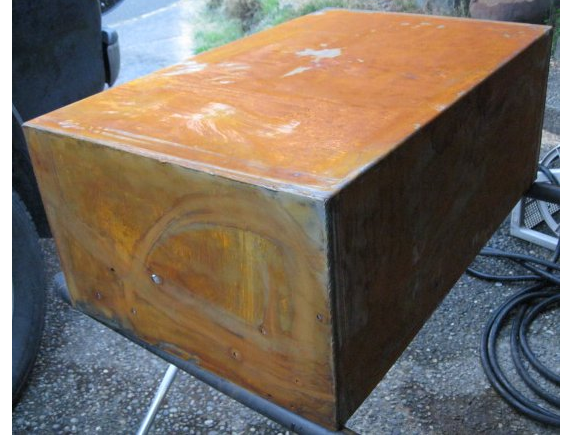
Water/vinegar mixture dried on bare metal. Don't panic!
