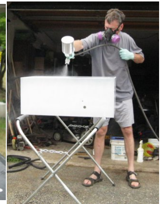
Shooting on the second coat of epoxy primer/sealer
